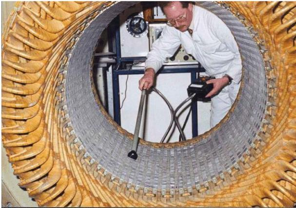
Fig. 4: Example of a corona probe test on a stator winding
