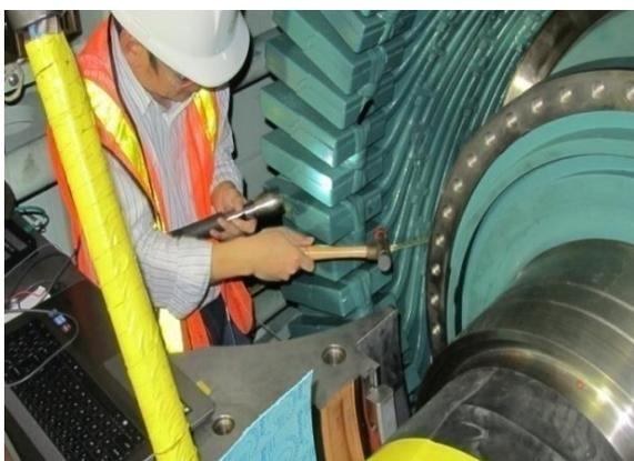
Fig. 7: Performing a bump test
