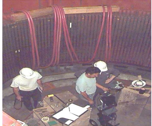
Fig. 10: Rated flux testing with power frequency
